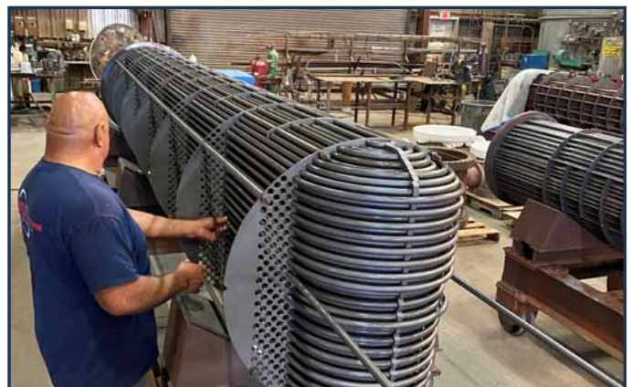
Curran installation of anti-foul coated tube; OD applications require precoating tubes prior to bundle fabrication.
