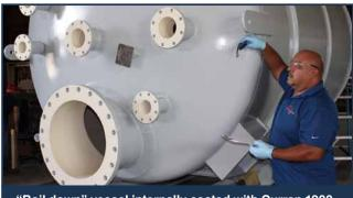
"Boil down" vessel internally coated with Curran 1200 novolac epoxy, externally painted with Carboline IOZ, epoxy and urethane system.
