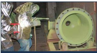
Curran coating tech using hot flock method to apply Chemours ETFE fluoropolymer to vessel head; coating is catayzed at 625F.
