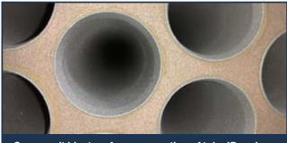
Curran grit blast surface preparation of tube ID and tubesheet yielded clean surface for coating.
