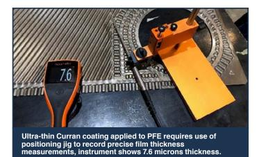
The coatings impart a low surface energy finish onto the substrate, improving release and promote sheer to minimize product attachment and nucleation sites. A wide collection of exchanger field trials ranging 15 to 60 months shows favorable results against uncoated exchangers in the same service.
