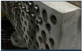
Full-length alloy liners used in a new fabrication replacement air cooler; client upgraded only primary inlet section where operating history showed tube corrosion was severe.
